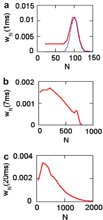
**Fig. 4.** Distribution of photons in blinking fluorescence calculated for various time intervals. Dashed line shows a Poissonian distribution. Average values of on- and off-interval are  $\tau_{on} = 3$  ms and  $\tau_{off} = 5$  ms.
