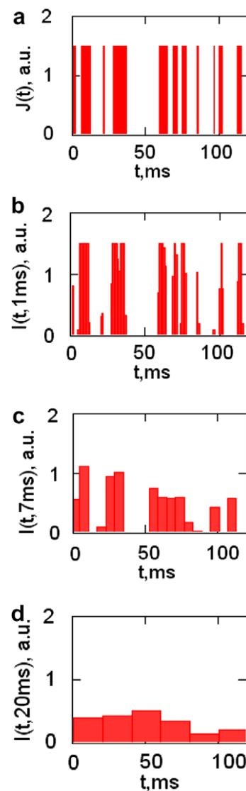
**Fig. 5.** Fluctuations of the fluorescence intensity at various values of bin time.
