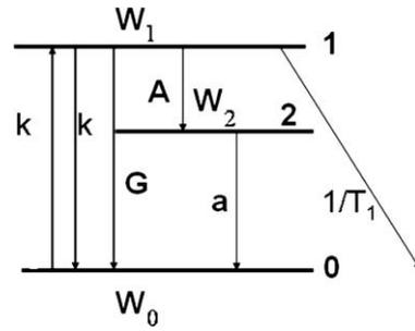
Fig. 1. Energy diagram for a three-level nanoparticle with “dark” state 2.
